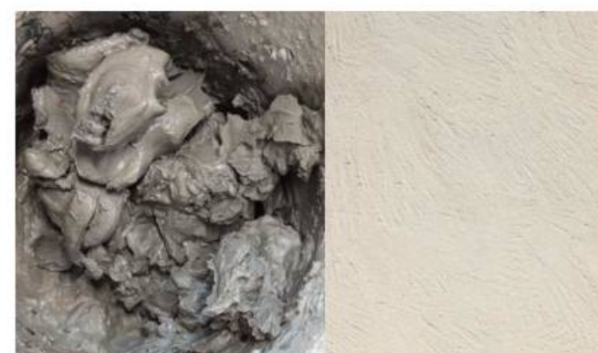
Clay plaster made from local sourced product
