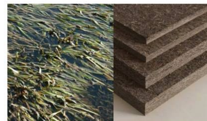
Acoustic panels made from eelgrass
